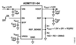
Figure 1. ADM7151-04 with  $V_{OUT} = 5 V$
