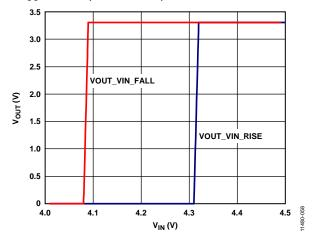
Figure 58. Typical UVLO Hysteresis,  $V_{OUT} = 3.3 \text{ V}$
