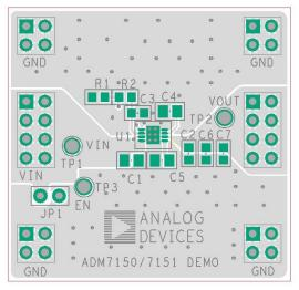
Figure 69. Example 8-Lead LFCSP PCB Layout
