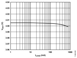
Figure 6. Output Voltage ( $V_{OUT}$ ) vs. Load Current ( $I_{LOAD}$ ), ADM7151-02,  $V_{OUT} = 4 V$
