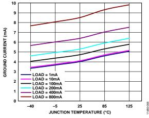
Figure 8. Ground Current vs. Junction Temperature (T<sub>J</sub>), ADM7151-02,  $V_{OUT} = 4 V$
