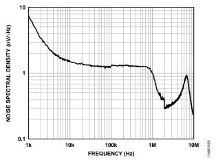
Figure 35. Output Noise Spectral Density, 1 kHz to 10 MHz, ILOAD = 10 mA
