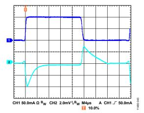
Figure 43. Load Transient Response,  $I_{LOAD} = 1$  mA to 100 mA,  $V_{OUT} = 5$  V,  $V_{IN} = 6.2$  V,  $CH1 = I_{OUT}$ ,  $CH2 = V_{OUT}$
