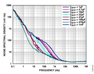
Figure 39. Output Noise Spectral Density vs. at Different  $C_{BYP}$ ,  $Load\ Current = 10\ mA$
