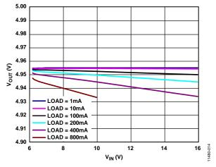
Figure 14. Output Voltage ( $V_{\rm OUT}$ ) vs. Input Voltage ( $V_{\rm INJ}$ , ADM7151-04,  $V_{\rm OUT} = 5~V$
