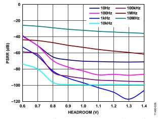
Figure 26. Power Supply Rejection Ratio (PSRR) vs. Headroom Voltage, ADM7151-02,  $V_{OUT} = 4 V$ , 400 mA Load
