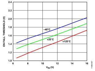
Figure 57. Typical EN Fall Threshold vs. Input Voltage (V<sub>IN</sub>) for Various Temperatures
