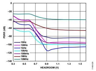
Figure 28. Power Supply Rejection Ratio (PSRR) vs. Headroom Voltage, ADM7151-04,  $V_{OUT} = 5$  V, 100 mA Load
