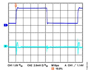
Figure 44. Line Transient Response, 2 V Input Step,  $I_{LOAD} = 800$  mA,  $V_{OUT} = 1.8 \text{ V}$ ,  $V_{IN} = 4.5 \text{ V}$ ,  $CH1 = V_{IN}$ ,  $CH2 = V_{OUT}$
