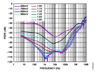
Figure 24. Power Supply Rejection Ratio (PSRR) vs. Frequency for Various Headroom Voltages, ADM7151-04,  $V_{OUT} = 5 V$ , 400 mA Load
