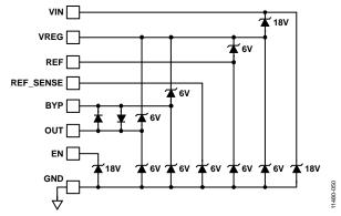
Figure 50. Simplified ESD Protection Block Diagram
