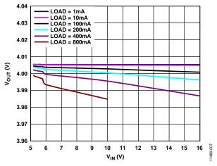
Figure 7. Output Voltage ( $V_{OUT}$ ) vs. Input Voltage ( $V_{IN}$ ), ADM7151-02,  $V_{OUT} = 4 V$
