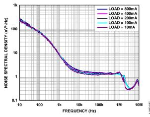
Figure 37. Output Noise Spectral Density at Different Load Currents, 10 Hz to 10 MHz
