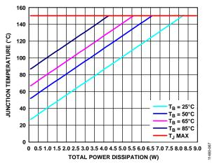
Figure 67. Junction Temperature vs. Total Power Dissipation for the 8-Lead LFCSP
