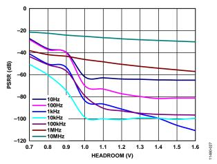
Figure 27. Power Supply Rejection Ratio (PSRR) vs. Headroom Voltage, ADM7151-02,  $V_{OUT} = 4 V$ , 800 mA Load
