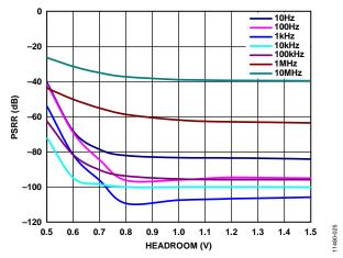
Figure 25. Power Supply Rejection Ratio (PSRR) vs. Headroom Voltage, ADM7151-02,  $V_{OUT} = 4$  V, 100 mA Load
