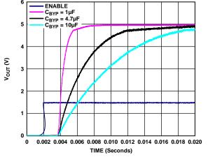
Figure 59. Typical Start-Up Behavior with  $C_{BYP} = 1 \mu F$  to 10  $\mu F$
