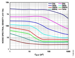
Figure 53. Noise Spectral Density vs. C<sub>BYP</sub> for Different Frequencies
