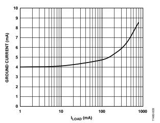
Figure 9. Ground Current vs. Load Current ( $I_{LOAD}$ ), ADM7151-02,  $V_{OUT} = 4 V$
