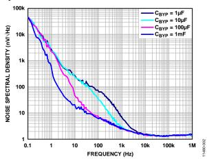
Figure 2. Noise Spectral Density (NSD) vs. Frequency for Various CBYP
