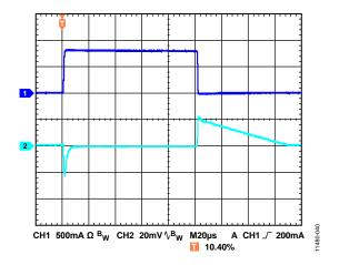
Figure 40. Load Transient Response,  $I_{LOAD}=1$  mA to 800 mA,  $V_{OUT}=5$  V,  $V_{IN}=6.2$  V, CH1 =  $I_{OUT}$ , CH2 =  $V_{OUT}$
