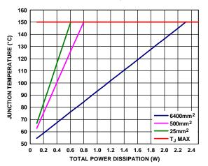
Figure 62. Junction Temperature vs. Total Power Dissipation for the 8-Lead LFCSP,  $T_A = 50^{\circ}\text{C}$
