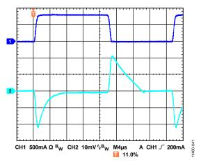
Figure 41. Load Transient Response,  $I_{LOAD}=10$  mA to 800 mA,  $V_{OUT}=5$  V,  $V_{IN}=6.2$  V, CH1 =  $I_{OUT}$ , CH2 =  $V_{OUT}$
