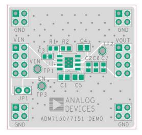
Figure 70. Example 8-Lead SOIC PCB Layout
