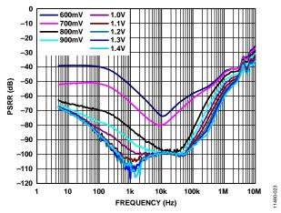
Figure 23. Power Supply Rejection Ratio (PSRR) vs. Frequency for Various Headroom Voltages, ADM7151-02,  $V_{OUT} = 4 V$ , 400 mA Load
