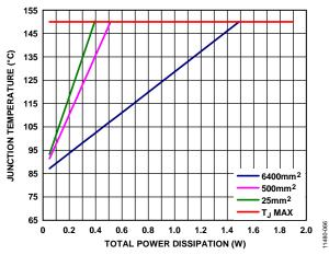
Figure 66. Junction Temperature vs. Total Power Dissipation for the 8-Lead SOIC,  $T_A = 85^{\circ}C$
