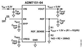
Figure 49. Typical Adjustable Output Voltage Application Schematic
