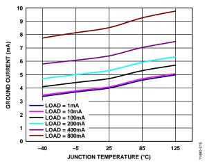
Figure 15. Ground Current vs. Junction Temperature (T<sub>s</sub>), ADM7151-04,  $V_{OUT} = 5 V$
