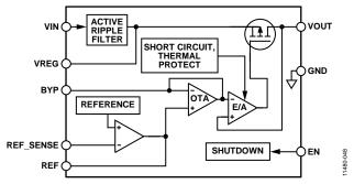
Figure 48. Adjustable Output Voltage Internal Block Diagram
