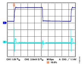
Figure 45. Line Transient Response, 2 V Input Step,  $I_{LOAD} = 800$  mA,  $V_{OUT} = 3.3$  V,  $V_{IN} = 4.5$  V,  $CH1 = V_{IN}$ ,  $CH2 = V_{OUT}$
