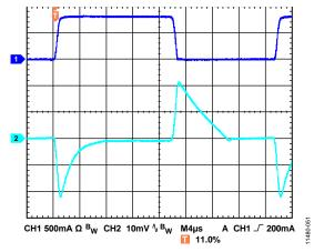
Figure 51. Output Transient Response,  $V_{OUT} = 5 V$ ,  $C_{OUT} = 10 \mu F$
