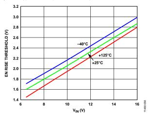
Figure 56. Typical EN Rise Threshold vs. Input Voltage  $(V_{\mathbb{N}})$  for Various Temperatures
