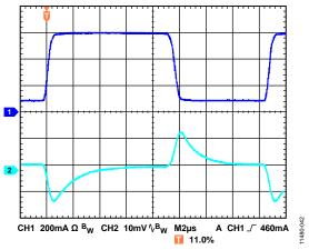
Figure 42. Load Transient Response,  $I_{LOAD} = 100$  mA to 600 mA,  $V_{OUT} = 5$  V,  $V_{IN} = 6.2$  V,  $CH1 = I_{OUT}$ ,  $CH2 = V_{OUT}$
