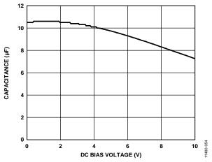
Figure 54. Capacitance vs. DC Bias Voltage
