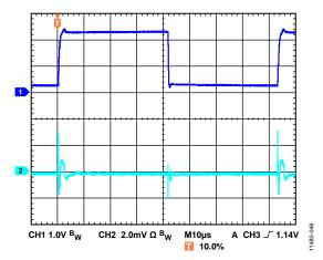
Figure 46. Line Transient Response, 2 V Input Step,  $I_{LOAD} = 800$  mA,  $V_{OUT} = 5$  V,  $V_{IN} = 6.2$  V,  $CH1 = V_{IN}$ ,  $CH2 = V_{OUT}$
