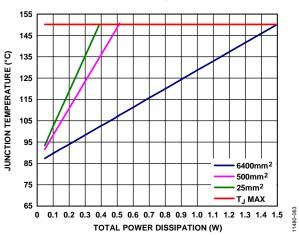
Figure 63. Junction Temperature vs. Total Power Dissipation for the 8-Lead LFCSP,  $T_A = 85^{\circ}C$
