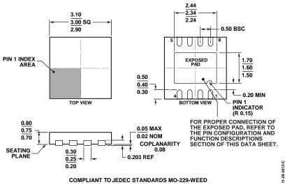
Figure 71. 8-Lead Lead Frame Chip Scale Package [LFCSP\_WD] 3 mm × 3 mm Body, Very Very Thin, Dual Lead (CP-8-11) Dimensions shown in millimeters
