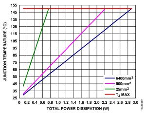
Figure 61. Junction Temperature vs. Total Power Dissipation for the 8-Lead LFCSP,  $T_A = 25^{\circ}C$
