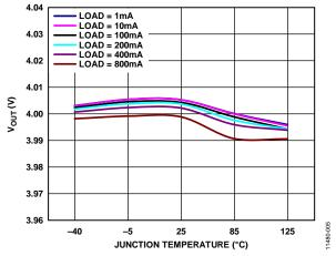
Figure 5. Output Voltage ( $V_{OUT}$ ) vs. Junction Temperature (T.), ADM7151-02,  $V_{OUT} = 4 V$
