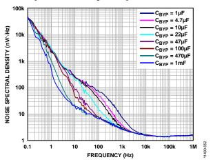
Figure 52. Noise Spectral Density vs. Frequency,  $C_{BYP} = 1 \mu F$  to 1 mF
