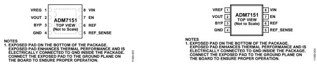
Figure 3. 8-Lead LFCSP Pin Configuration
