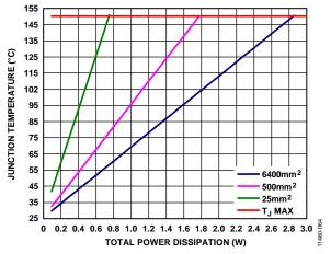
Figure 64. Junction Temperature vs. Total Power Dissipation for the 8-Lead SOIC,  $T_A = 25$ °C
