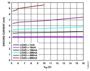
Figure 10. Ground Current vs. Input Voltage ( $V_{IN}$ ), ADM7151-02,  $V_{OUT} = 4 V$
